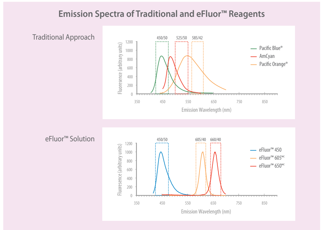
Figure 2: Emission spectra of traditional and eFluor™ reagents for the violet laser. Normalized emission spectra of the traditional fluorophores commonly used with the violet laser (top) versus the eFluor™ solution (bottom). The advantageous narrow emission spectra of the eFluor™ solution is evident when compared to the broad emission spectra and large spectral overlap of the traditional approach. The recommended collection filters for each fluorophore are indicated.
